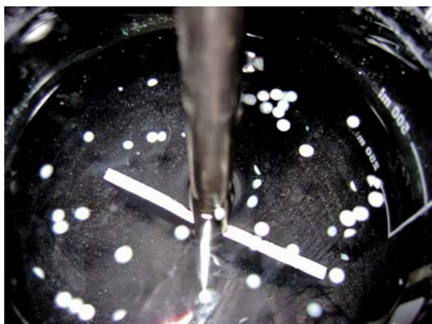
Figure 6. PEG pastilles floating in dissolution jar containing 0.1 N HCl.
